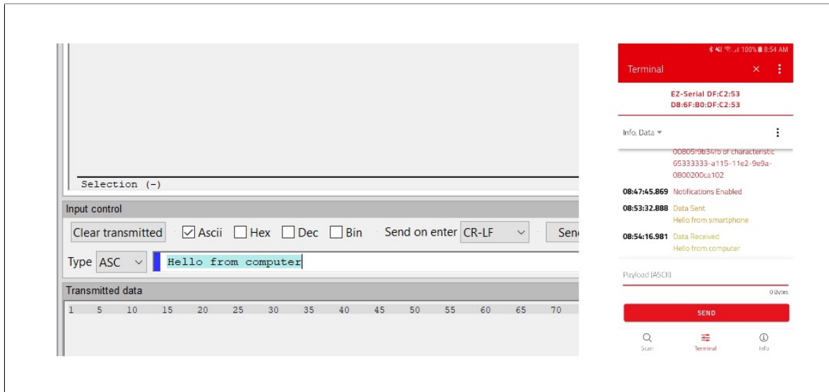
Figure 27: Sending a message via CYSP from the module to a smartphone
